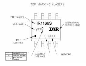
Order Information 8-Lead SOIC IR1166SPbF 8-Lead SOIC Tape and Reel IR1166STRPbF
