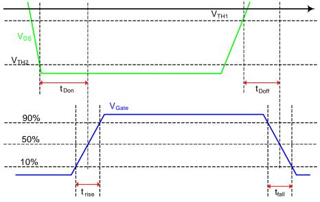
Fig. 15 - Timing Diagrams
