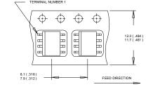
NOTES: 1. CONTROLLING DIMENSION : MILLIMETER. 2. ALL DIMENSIONS ARE SHOWN IN MILLIMETERS(INCHES). 3. OUTLINE CONFORMS TO EIA-481 & EIA-541.
