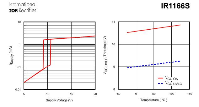
Fig 1. Supply Current vs. Supply Voltage
