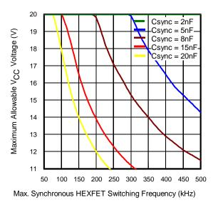
Fig 12. Max. V<sub>CC</sub> Voltage vs. Synchronous Rectifier Switching Freq, T<sub>J</sub>=125 C, T<sub>IC</sub> = 85 C, external  $R_{G}=2\Omega$ , 1Ω HEXFET Gate Resistance included
