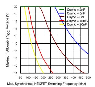
Fig 11. Max.  $V_{CC}$  Voltage vs. Synchronous Rectifier Switching Freq,  $T_J$ =125 C,  $T_{IC}$  = 85 C, external  $R_G$ =1 $\Omega$ , 1 $\Omega$  HEXFET Gate Resistance included
