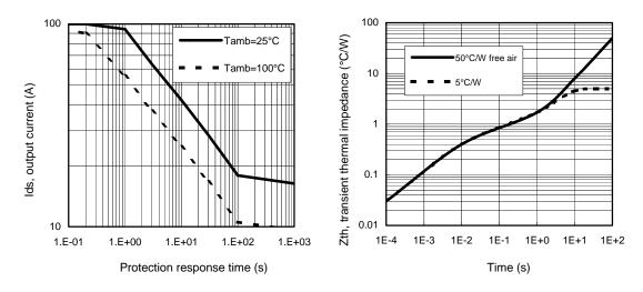
Figure 14 – Ids (A) Vs over temperature protection response time (s)/ Rth=60°C/W
