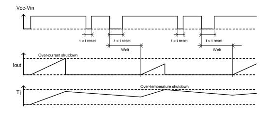
Figure 5 – Protection Timing Diagrams
