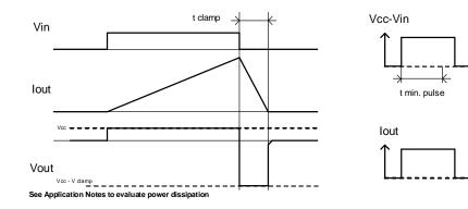
Figure 3 – Active clamp waveforms
