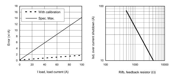
Figure 10 – Error (+/- A) Vs I load (A)
