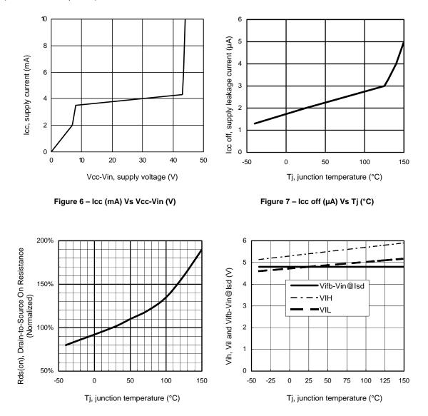
All curves are typical characteristics. Operation in hatched areas is not recommended. Tj=25°C, Rifb=500ohm, Vcc=14V (unless otherwise specified).
