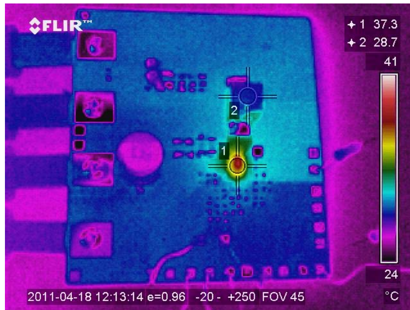
Figure 39: Thermal Image of the Board at 4A Load, Test Point 1 is IR3897, Test Point 2 is inductor
