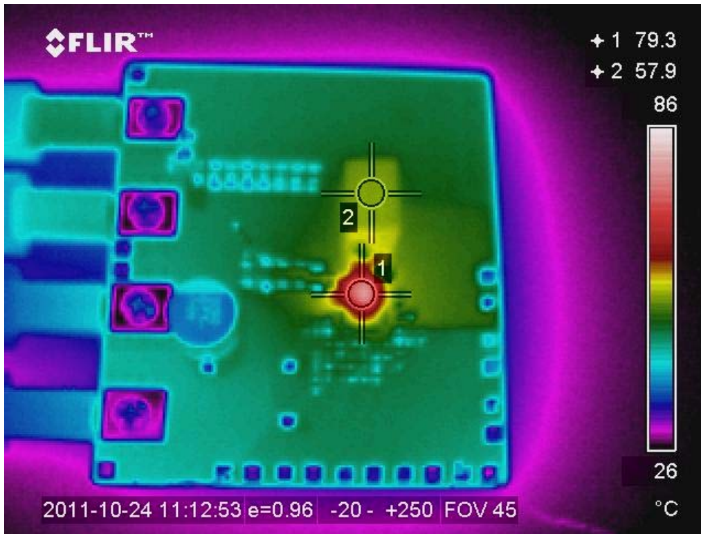
Figure 45: Thermal Image of the Board at 12A Load, Test Point 1 is IR3894, Test Point 2 is inductor
